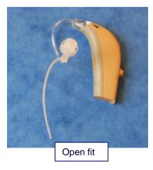
Some people who wear hearing aids use a custom made ear piece, others an open-fit. It is important to check the tubing and elbow for cracks, blockages and condensation.
