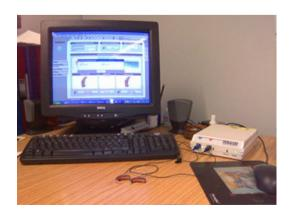
An appropriately powered digital hearing aid is programmed on a computer by an Audiologist to deliver the correct amount of amplification at each frequency to match the individual's hearing needs.
